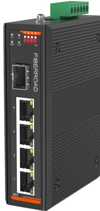
The industrial converter is equipped with rugged IP40 metal enclosure to ensure industrial operation in harsh environments where extreme low or high temperatures can be experienced. It is specially designed for outdoor and industrial applications such as city surveillance systems, smart manufacturing, etc. It is ideal for miniaturization and rapid deployment, provides users a cost-effective and highly reliable option.
