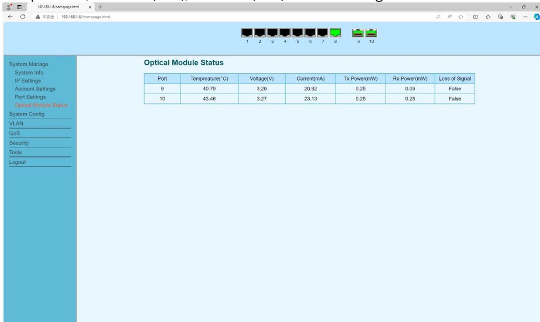
The screenshot displays a web-based network management interface. At the top, there is a navigation bar with icons for ports 1 through 10. Below this, a sidebar on the left contains a menu with options: System Manage, System Info, IP Settings, Account Settings, Port Settings, Optical Module Status (highlighted in red), System Config, VLAN, QoS, Security, Tools, and Logout. The main content area is titled "Optical Module Status" and contains a table with the following data:
