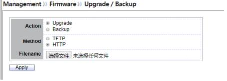
Figure 14-3 Upgrade Firmware through HTTP
