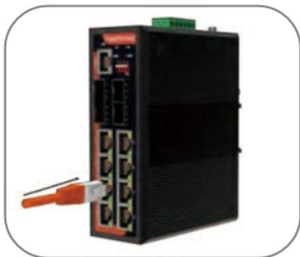
2. Connect the other end of the cable to an RJ-45 connector on the other device. The port LED turns on when the switch and the connected device have established a link. The port LED is amber while Spanning Tree Protocol (STP) discovers the topology and searches for loops. This can take up to 30 seconds, and the port LED turns green. If the port LED does not turn on:
