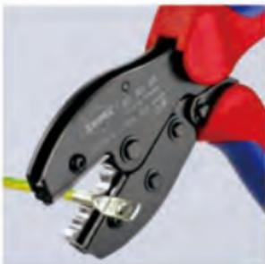
Figure: Crimping the Ring Terminal
