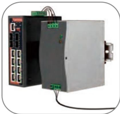
**Warning:** When used in Class I, Division 2, hazardous location, this equipment must be mounted in a suitable enclosure with proper wiring method for all power, input and output wiring that complies with the governing electrical codes and by the authority having jurisdiction over Class I, Division 2 installations.
