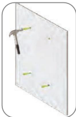
③ Insert the Screw Anchors
