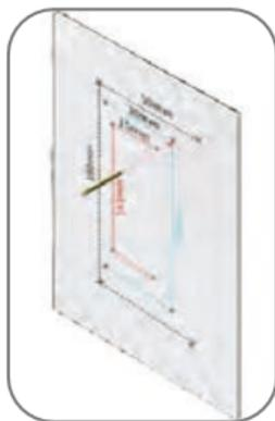
② Using 5mm Drill Bit to punch
