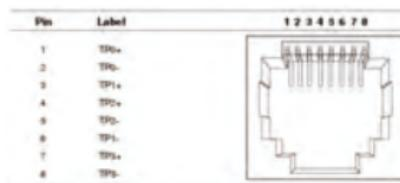
Figure: Ethernet Copper LAN Port Pinouts
