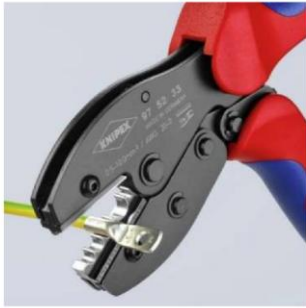
Figure: Crimping the Ring Terminal
