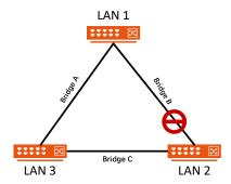
What happens if a link failure is detected? As shown in next figure, the STP process reconfigures the network so that traffic from LAN segment 2 flows through bridge B.
