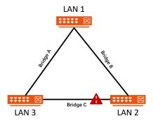
STP will determine which path between each bridged segment is most efficient, and then assign a specific reference point on the network. When the most efficient path has been identified, the other paths are blocked. In the previous 3 figures, STP first determined that the path through bridge C was the most efficient, and as a result, blocked the path through bridge B. After the failure of bridge C, STP re-evaluated the situation and opened the path through Bridge B.
