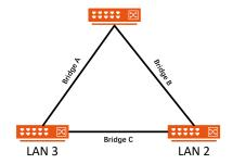
If STP is enabled, it will detect duplicate paths and prevent, or block, one of the paths from forwarding traffic. In the following example, STP determined that traffic from LAN segment 2 to LAN segment 1 should flow through bridges C and A since this path has greater bandwidth and is, therefore, more efficient.
