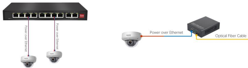
Figures 2 & 3, PoE Switch and PoE Media Converter
