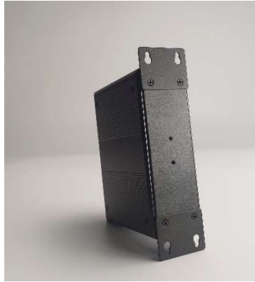
Figure 13 Remove the wall-mounted metal plate from the switches and re-install
